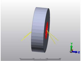
The stand consists of the yellow struts supporting the hub. The bottom of the struts are fixed to the ground. The wheel is given an initial velocity equal to 55 mph. The vertical position, or y, is plotted as time goes on.
