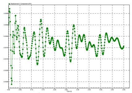
This graph shows the position of the center of the hub while the wheel is spinning. Note there is a small amount of variation in position. Also note that due to gravity, the position is almost all negative. This graph is shown for only ½ second which allows for 3.58 revolutions of a 43 inch tire.
