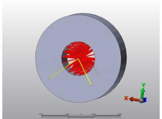
Note small brown arrow at about 4 O'clock position. There is one of these on each side and shows where a mass of 8 ounces has been placed on the wheel rim to cause an out of balance condition. We will rotate this model at the same 430 rpm that the balanced model was spun.
